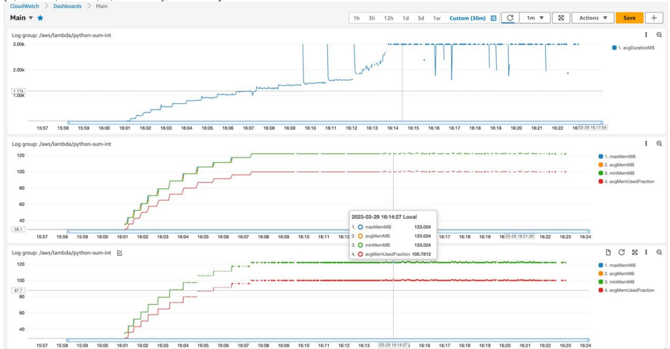
Fig. 2. Memory usage and average duration of calls to the sum of integer function on AWS Lambda. The function was called with n \in \{0, 200'000, 400'000, \dots, 5'000'000\} , with 40 requests for each n .
